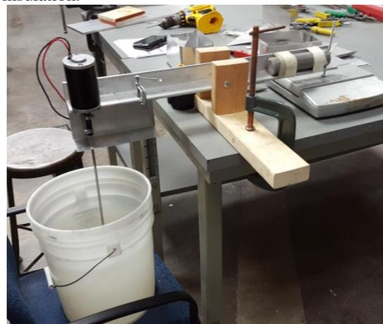
Fig. 6 CIM Motor Testing
