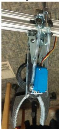
Fig.6. Vertically mounted claw
