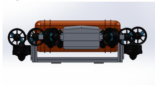
Fig. 4. Frame, thruster, and hull rendering for Paco 2.0
