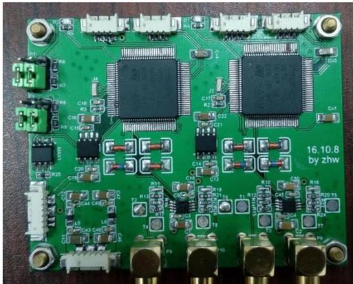
Fig 6: hydrophone signal processing system
