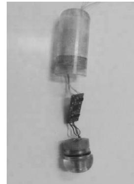
Fig 7. Disassembled depth sensor.
