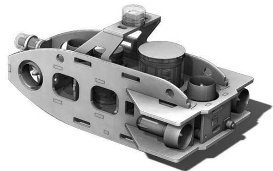
Fig 1. A SolidWorks render of MSU AUV.
