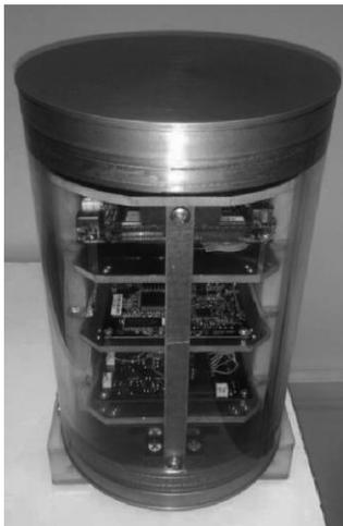
Fig 5. On board electronics inside housing.
