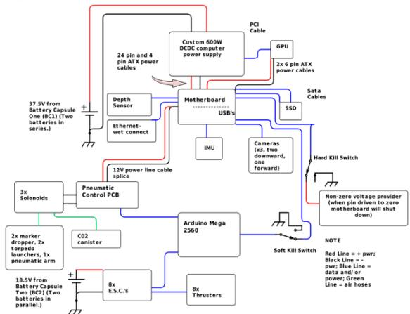
Fig. XX provides simplified details regarding the various connections running to and within the main electronics capsule.
