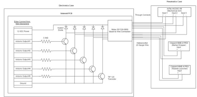
Fig. WW. Above contains the wiring diagram and necessary parts to build the pneumatics control PCB.
