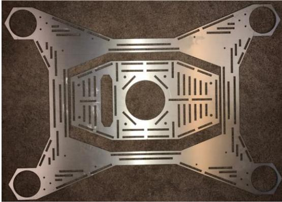
Fig 4: Main and belly frame with guide grooves
