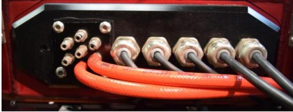
Fig. 8: Lateral IO port with nonpermanent cable glands and pneumatic hose barbs
