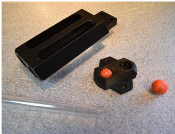
Fig.9: Torpedo launcher (left) and dropper and payload (right)
