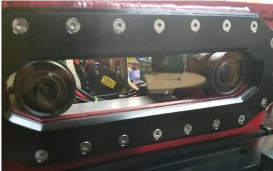
Fig. 13: Forward - stereo vision cameras
