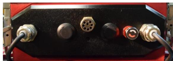
Fig. 7: Back IO port with kill switches, thruster cables, and ethernet tether
