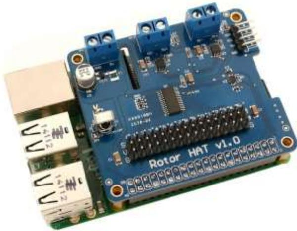
Fig 3. Our Raspberry Pi with top-mounted Rotor Hat Servo Controller.
