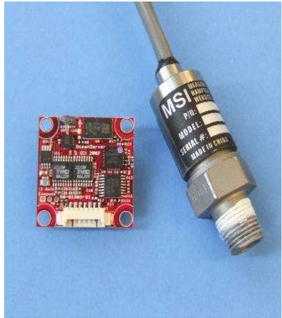
Fig 2. OS-5000USD Compass and MSI Pressure Transducer
