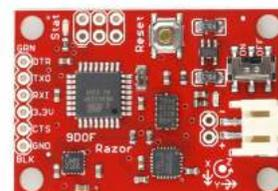
Figure 8. Razor 9DOF IMU
