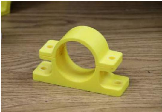
Figure 2. 3D Printed Mounts for Cameras
