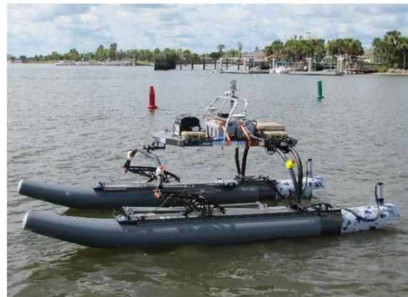
Figure 1 Minion ASV undergoing testing
