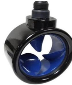
Figure 3: Rim Driven Propeller (RDP)
