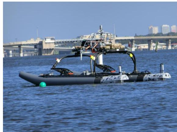
Figure 10 Minion testing its hydrophone array in the Halifax River
