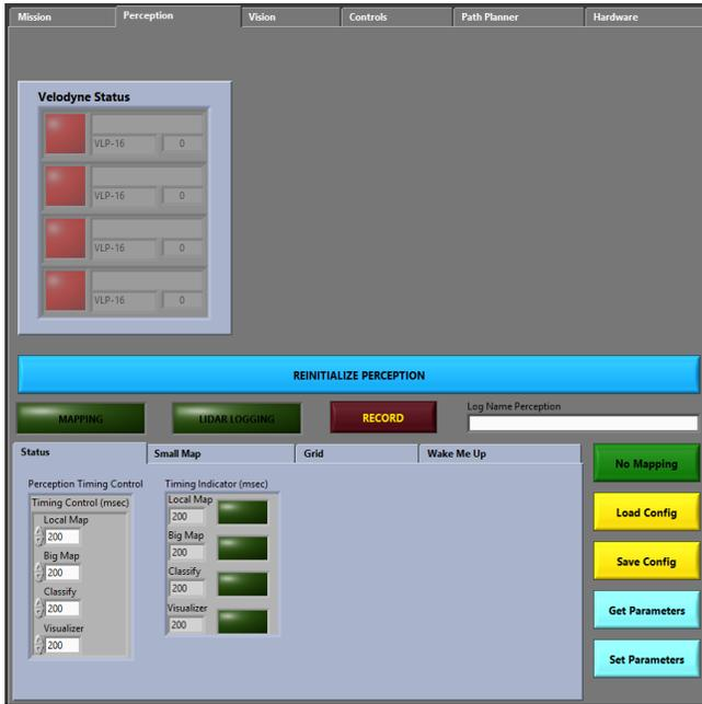
Fig 9. Communicates and sets perception settings from the Ground Station to the Perception module.
