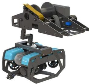
Fig 5. BlueROV2, Anchor, and deployment showing swing-arm.
