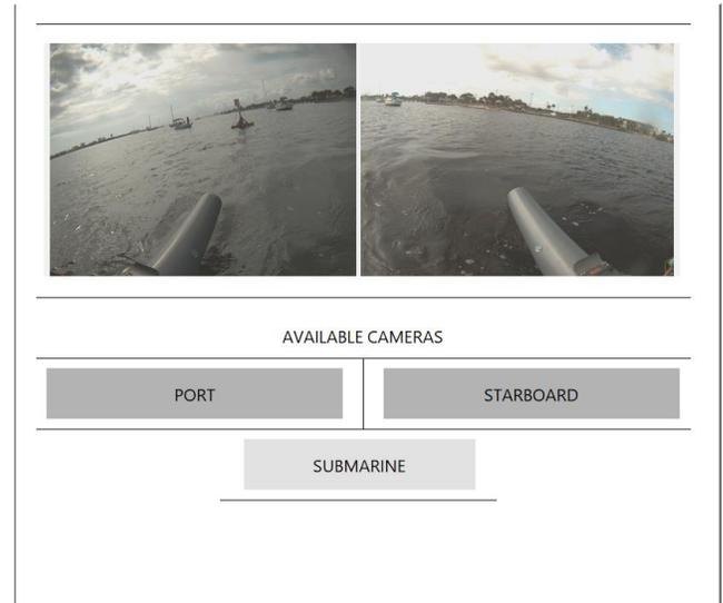
Fig 5. The Cameras tab of the MinionTab UI that displays the boat, submarine, and turret cameras.
