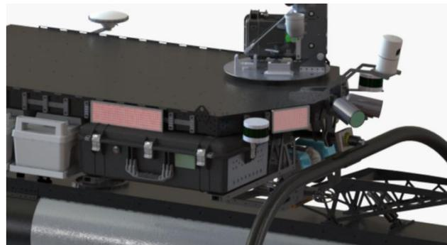
Fig 15. Render depicting indicator panel modules mounted to the starboard side of the Minion ASV.
