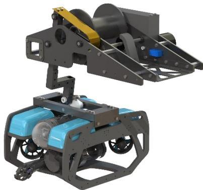
Fig 1. The Submarine Deployment System with the BlueROV2, Anchor
