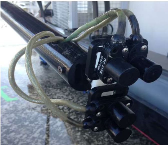
Fig. 3. Physical Hydrophone Configuration for Acoustic Data Acquisition System
