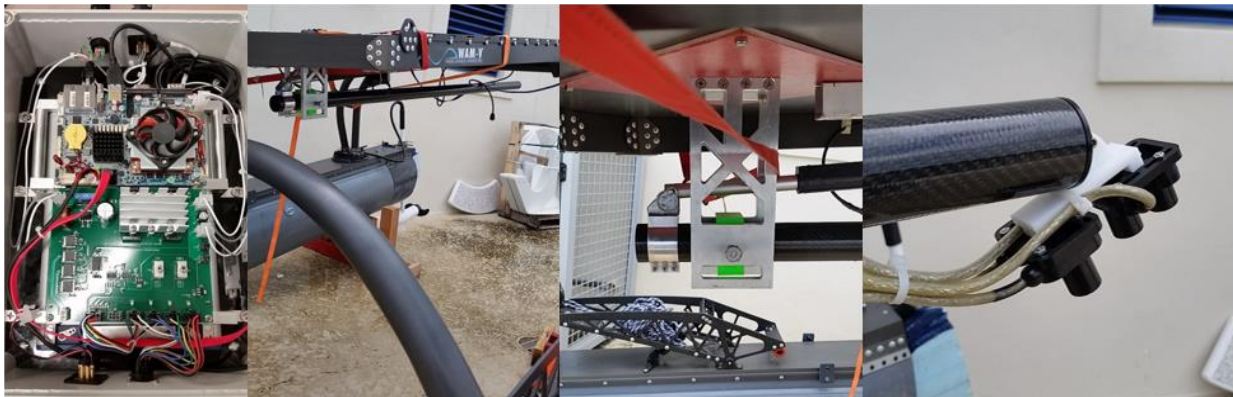
Figure 10: USBL positioning system acquisition and processing electronics (left); Automated launch and recovery system (center left); Actuation system for automated deployment and recovery of USBL positioning array (center right); USBL positioning array with horizontal and vertical baselines (right).
