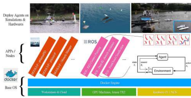
Fig. 1: We proposed an autonomous surface/underwater system with modular design and is compatible both with ROS and MOOS. The system is capable of running in real robots, minitured robots and simulations. The capability of running in multiple platforms provide us better tools to develop deep learning algorithms.
