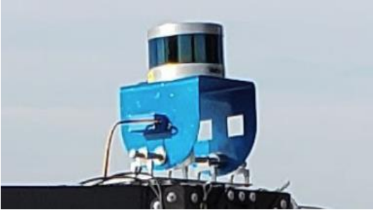
Figure 2: LiDAR Mount bracket shown in blue. It allows the system to pivot from level to 13.6 degrees down.
