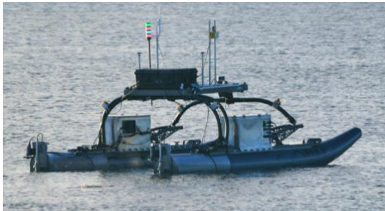
Figure 1: Image of ODUSSea WAM-V on starboard side with view of motor shafts.
