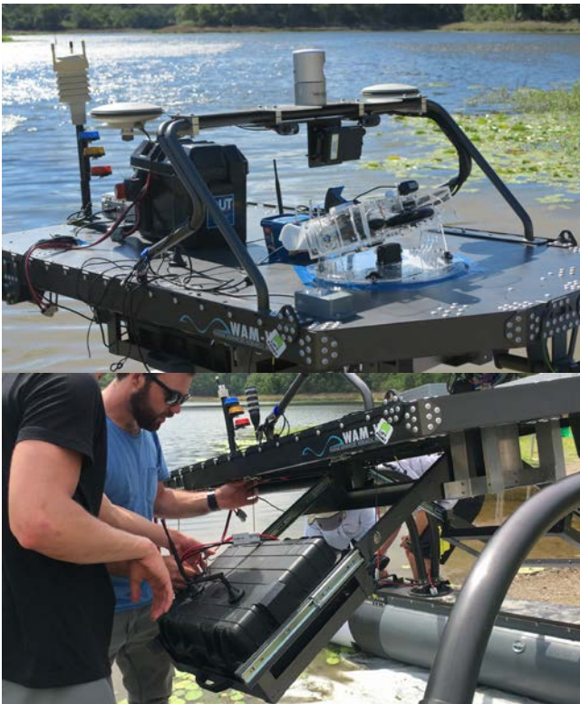
Fig 2. Top: The payload tray showing the sensor frame with Velodyne LiDAR, cameras, GPS and radar attached. Also visible is Gusto, the automated racquetball launcher and the Vaisala weather station. Lower: The sliding tray mechanism to allow shore-side access to the computing boxes.
