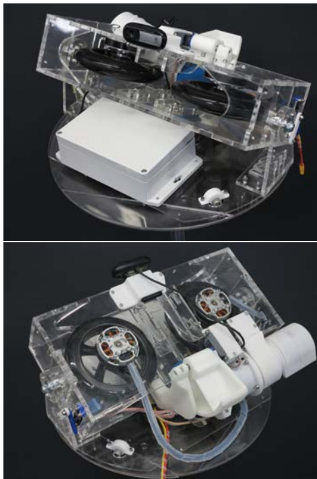
Fig 3. Gusto – the automated racquetball launcher for the “Detect and Deliver” task. (Top) Front view showing camera and electronics box, (Lower) rear view showing the automated ball feeder.
