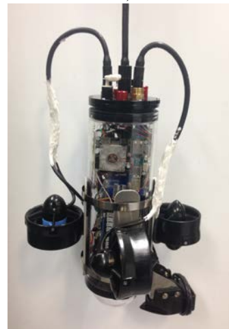
Fig 4. George – the autonomous underwater robot to provide imagery and symbol detection for the “Underwater Survey” task.
