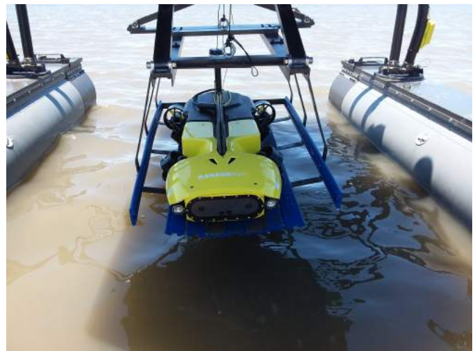
Fig. 5: The Autonomous Underwater Vehicle (AUV), called Thunder4 , used for the underwater ring challenge. This is a tethered hybrid (ROV/AUV) version of the RangerBot AUV.
