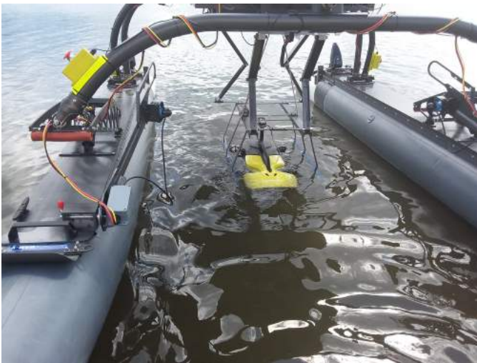
Fig. 6: The Thunder4 AUV in the lowered position ready to drive out of the lifting cradle.
