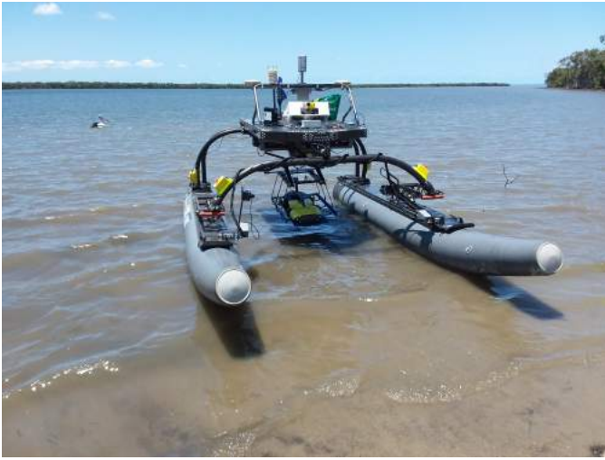
Fig. 2: The complete Autonomous Marine System (AMS) showing the ASV (aka Bruce), the AUV (aka Thunder4) and the racquetball launcher (aka Gusto).
