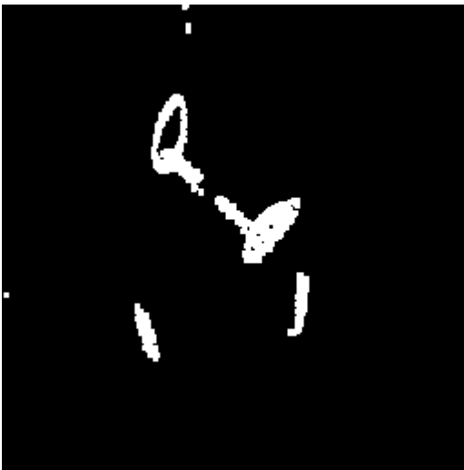
Fig. 13: The underwater ring segmentation process required multiple iterations. The red pole was not able to be directly segmented out without losing the rings, so is removed using binary subtraction.
