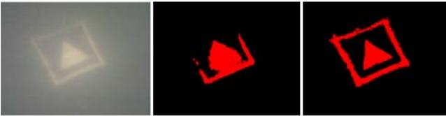
Fig. 15. Binarization of an underwater image a) original image b) Constant thresholding c) Niblack binarization method
