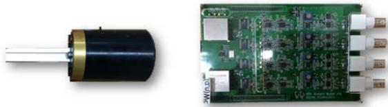
Fig. 2. Hydrophone and preprocessor used for acoustic sound detection
