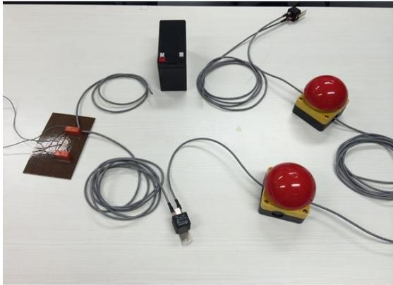
Figure 5: Actual setup of fail-safe circuit
