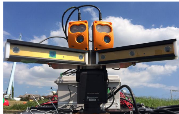
Figure 13 - Final Configuration of the Vision System
