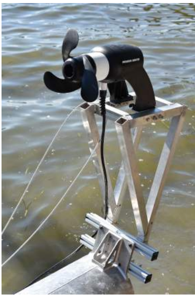
Fig. 3. The motors, shown in the out-of-water configuration which allows the vehicle to be brought into shallow areas without damaging the propellers.
