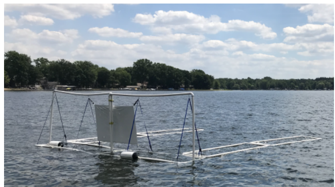
Fig. 9. The PVC dock used to test the docking task maneuverability and image recognition.
