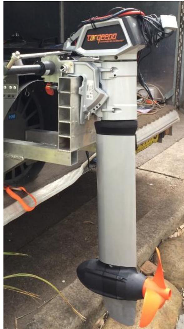
Figure 3: Propulsion unit with electric motor, linear actuator and motor mount.
