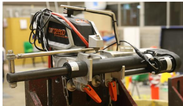
Figure 1: The linear actuator (foreground) attached to the electric outboard motor. An external encoder is mounted to the top of the outboard motor.
