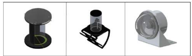
Fig. 14. Design iterations of the cameras housing with the final design on the right.
