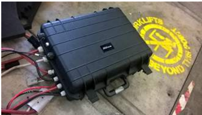
Fig. 13. Power Distribution housed in a waterproof case.
