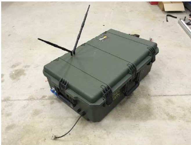
Fig. 12. Computer hardware housed in a Storm iM2950 waterproof case.
