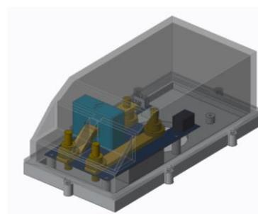
Figure 7 Thrust Current Transducer Design
