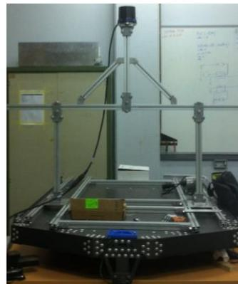
*Figure 4: The Antenna Mast mounted to the Modular Rail System allowing adjustment to position without drilling new mounting holes in the WAM-V payload tray.*
