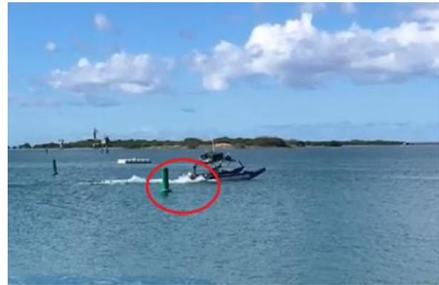
Figure 13: Large turbulence caused by inefficient floatation pod design.
