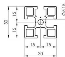
*Figure 3: System 30, T-Slot Aluminium extrusion profile allows standard fasteners to be used when assembling and attaching to the Modular Rail System.*
