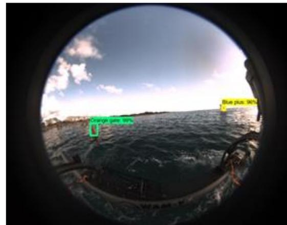
Figure 11: Object identification using a convolutional neural network where the bounding box and probability is shown.
