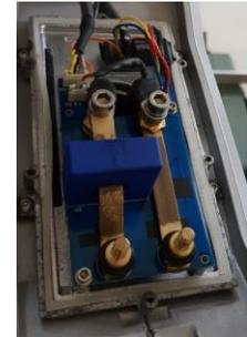
Figure 8 Thrust Current Transducer Implementation
