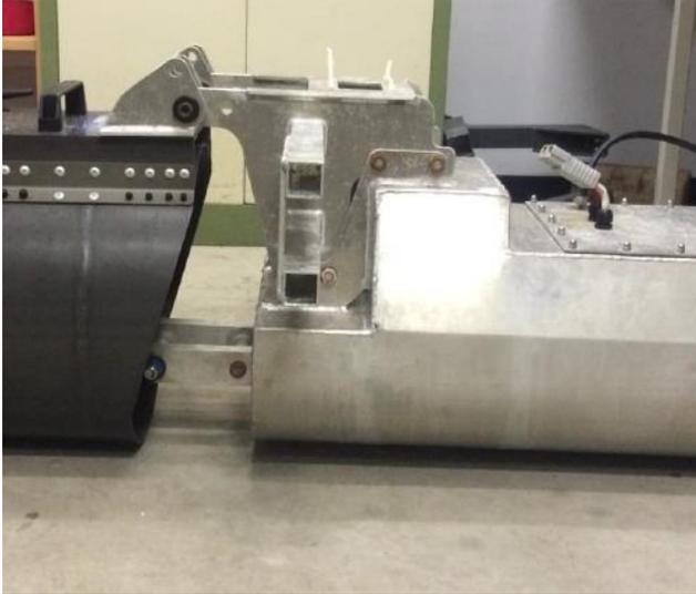
Figure 5: Floatation pod design used in the 2016 competition. A large void is present between the rear of the WAM-V pontoon and the floatation pod which produced large drag forces when underway.
