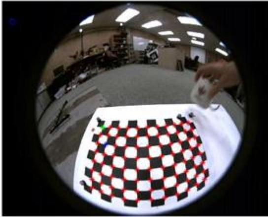
Figure 12: Camera calibration using VICON motion capture equipment.
