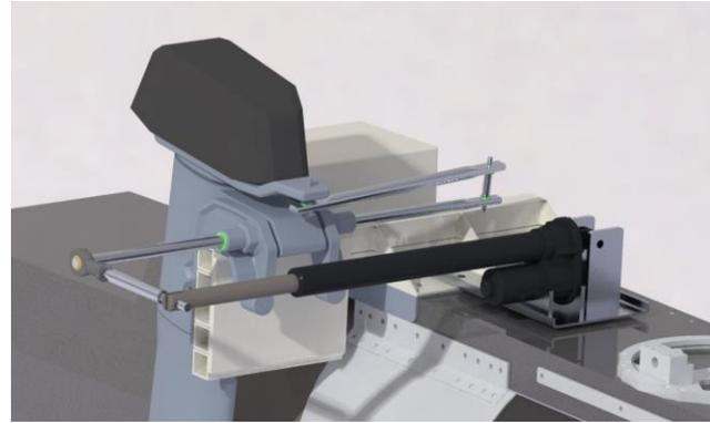
Figure 6 Linear-Actuator Based Steering System
