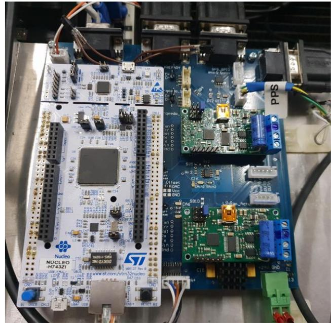
Figure 9 Signal Conditioning and Interfacing Board
