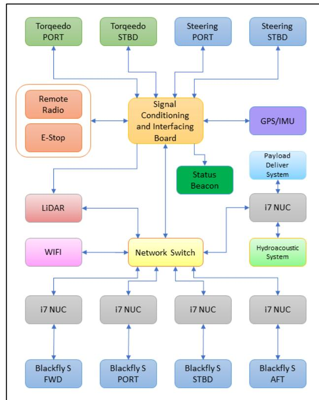
Figure 10 Computer System Block Diagram
