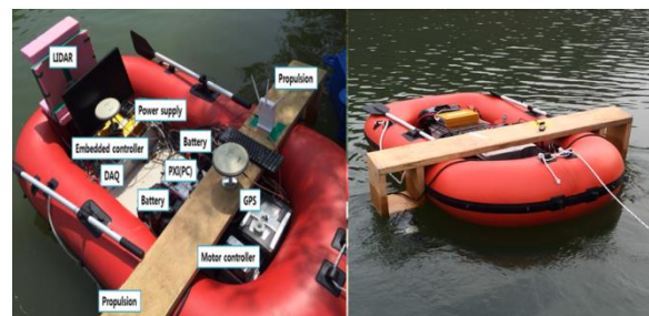
Figure 17 On-site test in Doohyun Reservoir using a rubber boat
