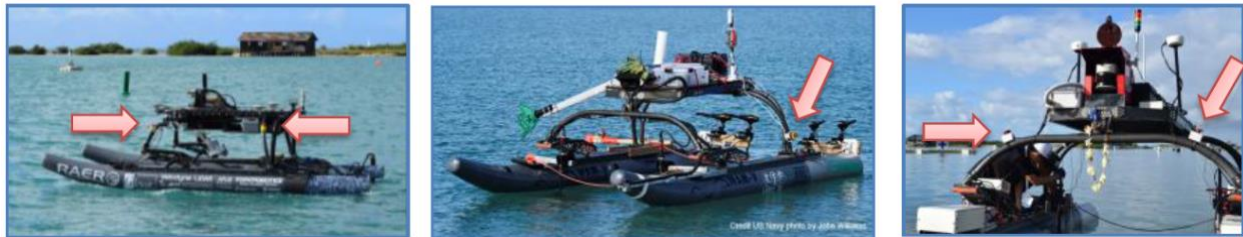
Figure 21: Examples of Kill Switch Placement
