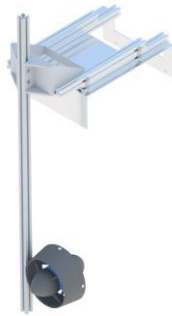
Figure 14: A computer assisted drawing of front thruster mount design, with a BlueROV thruster attached to the aluminum extrusion.
