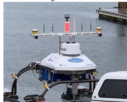
Figure 4: The Visual Indicator System, constructed from a weatherproof RGB light strip wrapped around a housing, hosting the electronics, allowing a wind sensor to be mounted on the top of the beacon.
