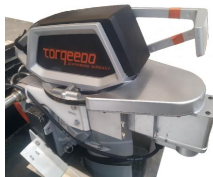
Figure 7: Steering module using a toothed pulley system controlled by a servo.
