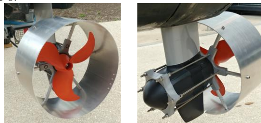
Figure 8: A custom manufactured shroud installed on Torqeedo thrusters, inspired by the manufacturers design.
