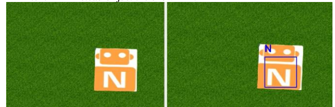
Fig 11. The UAV attempting to recognize the letter “N” shown in the image. The left is the raw footage captured while the right is the image after text detection and recognition. The UAV can correctly predict the text.
