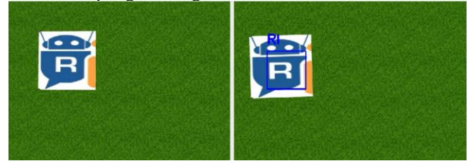
Fig 10. The UAV recognizing the text from the onboard camera. The left image is the raw footage, and the right image is the image after processing and analyzing. The UAV predicts the image contains the text “RI” instead of just the shown “R.”
