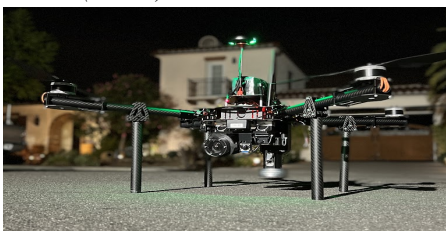
Fig 5. Full system view of assembled UAV. Note the camera positioned at the front of the perception rail.
