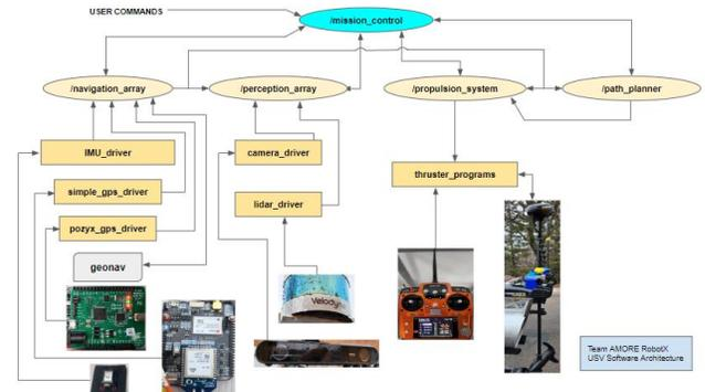
Fig 12. Autonomous software architecture implemented on the USV.
