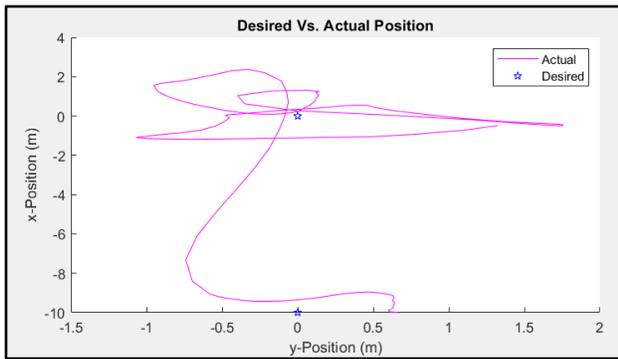
Fig 16. When the USV is given a pose to station-keep at, it first navigates to that location and then attempts to hold its position. This figure shows the desired position as a blue star and the USV x and y location as a pink line.
