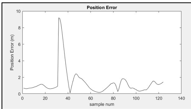
Fig 17. As the USV navigates to a specific pose, error in position should decrease. This means that the magnitude of the error signal should decrease as the sample number increases. .
