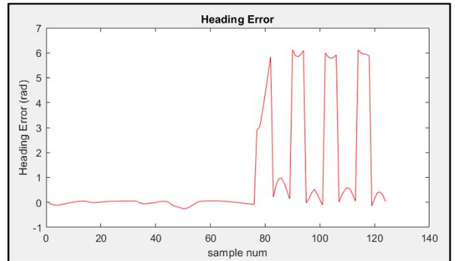
Fig 19. As the USV navigates to a specific pose, error in heading should decrease. This means that the magnitude of the error signal should decrease as the sample number increases.
