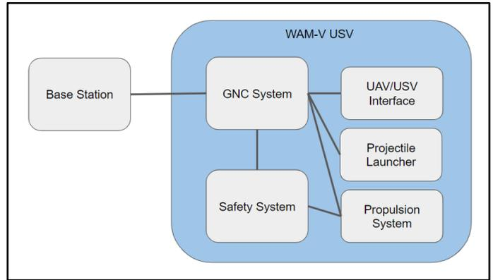
Fig 2. The top-level system architecture for the USV includes the GNC System, Safety System, UAV/USV interface, Propulsion System, and Projectile launcher. The GNC System will also interact with a Graphical User Interface.
