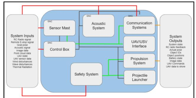
Fig 3. The mid-level system architecture for the USV includes more details about the interactions between different systems. It also provides information about expected inputs and outputs. The red lines represent USV system input, green lines represent electrical power transfer, black lines represent control data, and orange lines represent USV system output.
