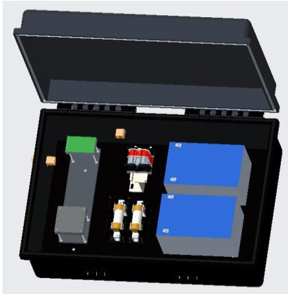
Fig 6. CAD drawing showing the layout of the GNC Battery Box.
