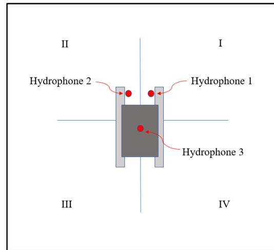
Fig 10. The acoustics system implemented on the boat will have three hydrophones. Two for determining direction and one for determining amplitude. The Roman Numerals I-IV represent the quadrants that a noise could originate from.
