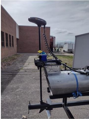
Fig 4. The USV's propulsion system includes 12V Minn Kota PowerDrive thrusters, 3D printed potentiometer assemblies, and custom aluminum mounting brackets.
