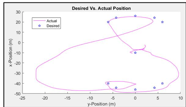
Fig 20. In waypoint following the USV must attempt to navigate through a series of waypoints. The waypoints are marked as blue stars and the actual USV path is represented as a pink line.
