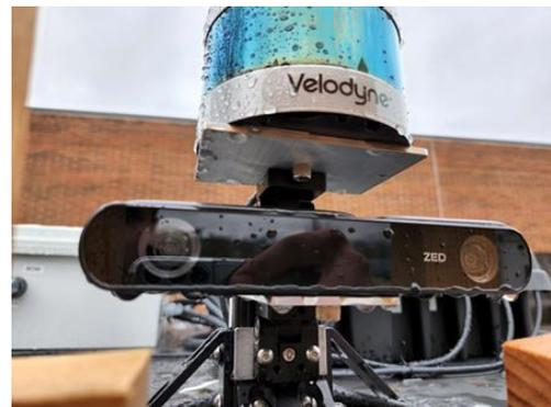
Fig 8. The vision system implemented on the USV is composed of a ZED 2i Stereo Camera and Velodyne VLP-16 LiDAR.
