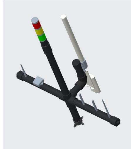
Fig 7. The USV has an Antenna mast located on its top tray. This mast also supports the lightstack. .
