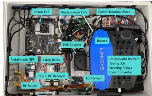
Fig 5. The Primary GNC Box holds the majority of the electronics onboard the USV.
