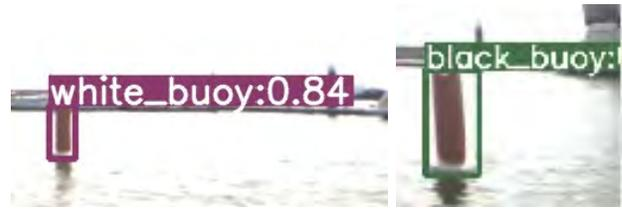
Fig. 25: Red buoy wrongly identified as a white buoy (left) and black buoy (right).
