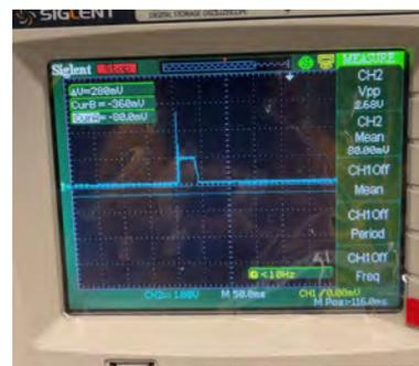
Fig. 29: High inrush current through the inverter.
