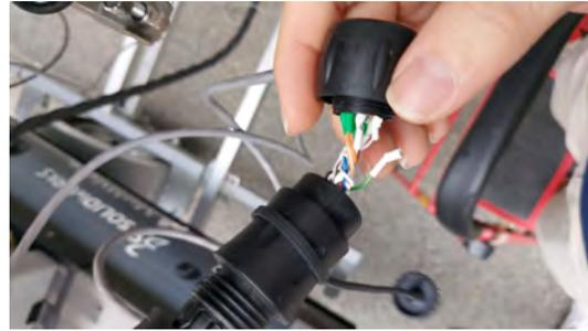
Fig. 21: Broken Soriau UTS Series connector.
