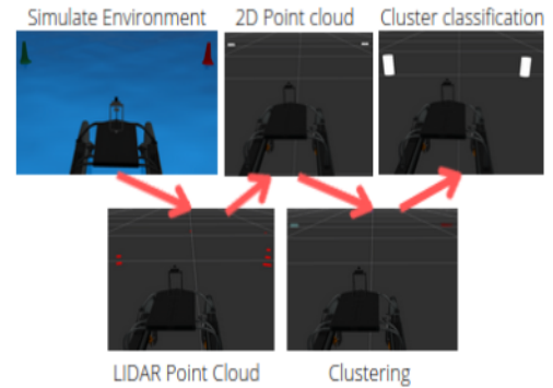
Figure 8: The complete Perception processing algorithm: 1) Point Clouds projection from 3D space to 2D space. 2) Grouping of agglomerations. 3) Cluster classification
