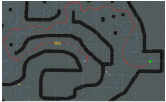
Fig. 5. The NaviGator ASV's real-time ROS-integrated RRT algorithm being run on an arbitrarily drawn, complicated occupancy grid
