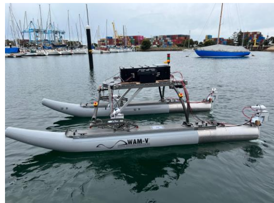
Fig 15. USV undergoing on-water testing at the Royal Yacht Squadron of South Australia. The swerve drive, which consists of the four outboards and the associated turning systems, met all performance targets.
