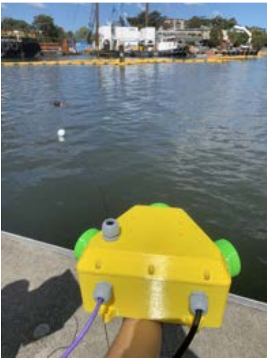
Fig. 7. Testing of the camera module with small floats
