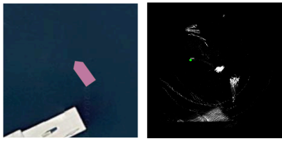
Fig. 13. Occupancy grid with overhead view and visual noise of data from moving fishing vessel
