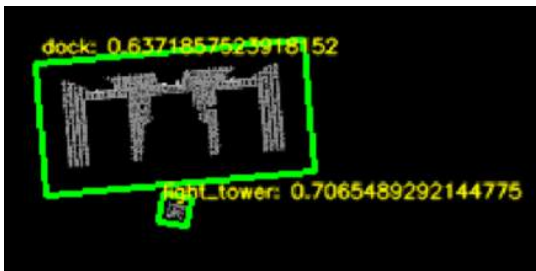
Fig. 9: LiDAR BEV detection (in simulation).
