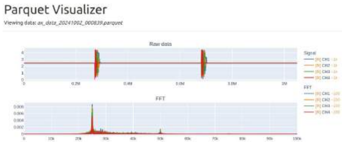
Fig. 5: Interactive visualization of acoustic data.
