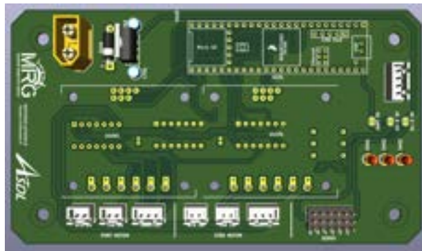
Fig. 8. Custom Motor controller PCB. Implements WigWag control of Elco EP-5 motors through digital potentiometers.
