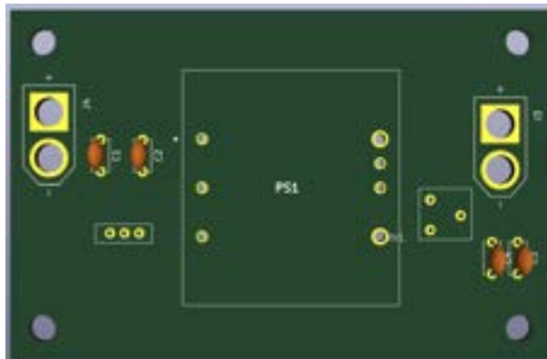
Fig. 9. Custom Buck Converter PCB. Regulates battery voltage to supply WAM-V's network switch
