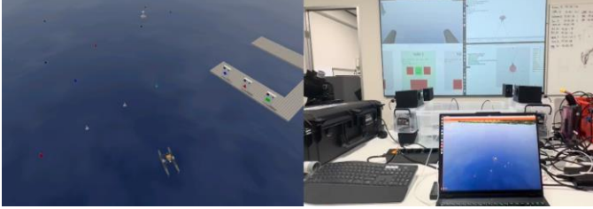
Fig. 16: VRX environment for RobotX tasks(left), Hardware In the Loop Simulation setup(right)
