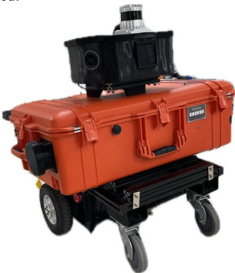
Fig. 19: UGV with sensor box and system box
