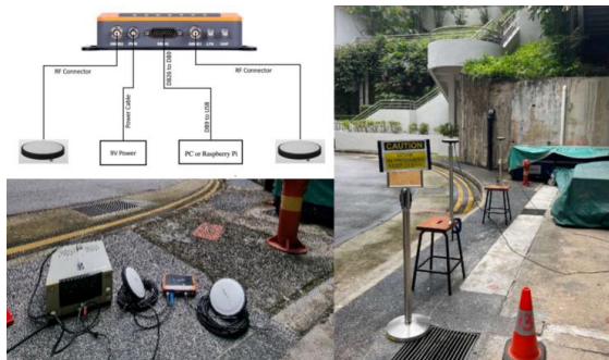
Figure 4: Connection diagram and testing of GPS hardware.
