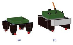
Figure 1.(a) Hull design of first generation PENSHIP, (b) New hull design of second generation PENSHIP
