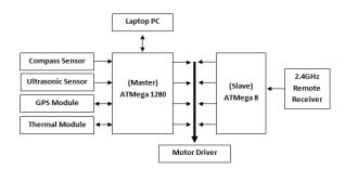
Figure 4. Block diagram of main control board
