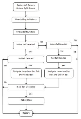
Figure 14. Ball detection algorithm of PENSHIP
