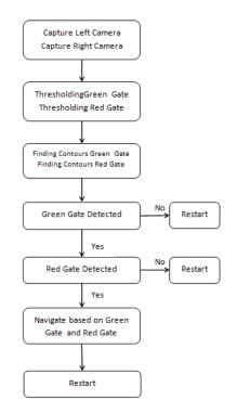
Figure 13. Gate detection algorithm of PENSHIP
