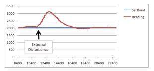
Figure 10. PID controller experiment result
