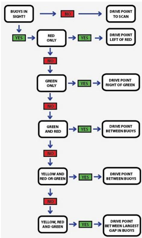
A proportional-derivative control law is used to determine how the vessel drives to a specified drive point. Using a local, vehicle-based coordinate frame, the distance and angle to the point of interest is calculated. As the vehicle approaches the drive point, it will begin to slow down. The turning component commanded from
