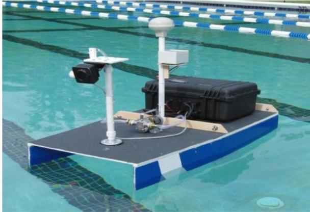
Seagle 4.0 is a small electrically propelled pontoon boat that is differentially driven by two VideoRay motors from the VideoRay PRO 4 ROV. Seagle 4.0 is 36 inches long, 24 inches wide and 14 inches high (excluding the payload and GPS mast). Where appropriate, Seagle 4.0 incorporates commercial, off-the-shelf components to help ensure reliability.
