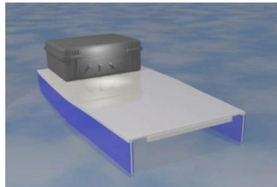
Figure 2 shows the initial design created in CATIA. The plywood keels also provide a secure structure for the thrusters. The Styrofoam and plywood are joined using Gorilla Glue brand polyurethane adhesive. The deck is joined to the pontoon assemblies with wood screws, creating a lightweight structure that can be easily assembled and disassembled. The pontoon assemblies and main deck are coated with glass microballoon filled epoxy to make them tougher and more resistant to water.
