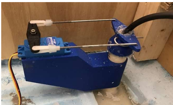
Figure 4: The azimuth assembly, which protrudes through the bottom of the hull to the Blue Robotics T200 thrusters.
