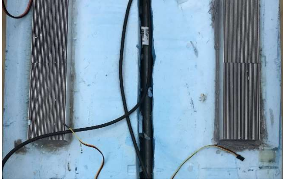
Figure 3: The two radiators that transfer internal heat to the water below the vessel, and the steel rods used as ballast in the bottom of the hull.
