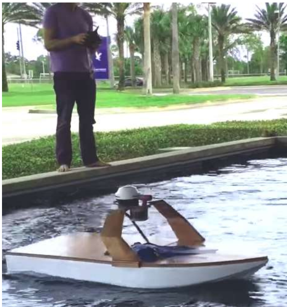
Figure 1: The Double Precision ASV during a test in the ERAU Henderson Welcome Center pond.
