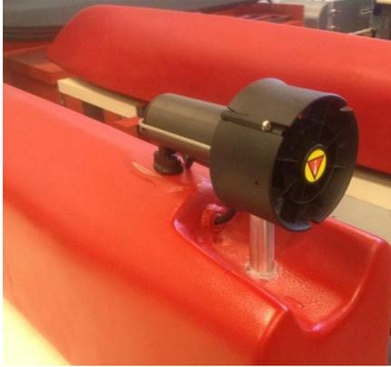
**Figure 3: New Seabotix thrusters mounted.**
