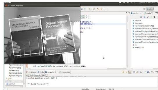
Figure 6: Feature detection using the SURF algorithm.
