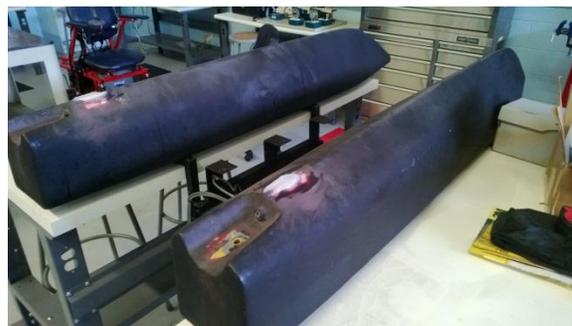
**Figure 2: V-BASS hull getting prepped for mounting new Seabotix thruster mounts**
