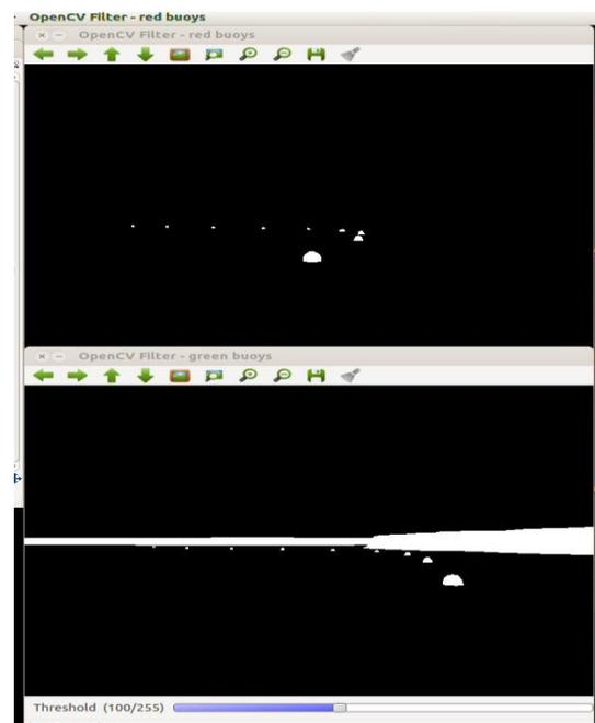
**Figure 9:** Threshold image of vehicle entering into buoy channel.
