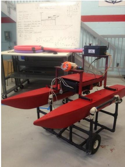
**Figure 1: The acclaimed V-BASS: Vision-Based Autonomous Surface Ship platform.**
