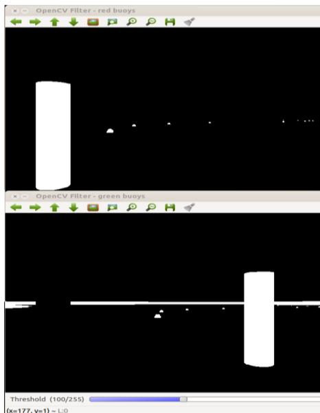
**Figure 8:** Threshold image of vehicle approaching end of speed gate.
