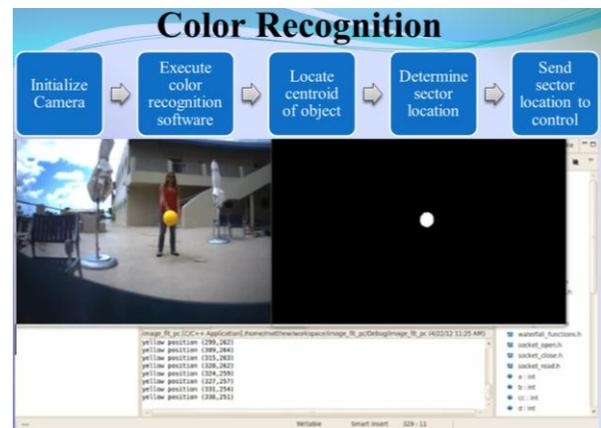
Figure 5: Color tracking calibration using OpenCV for image thresholding.
