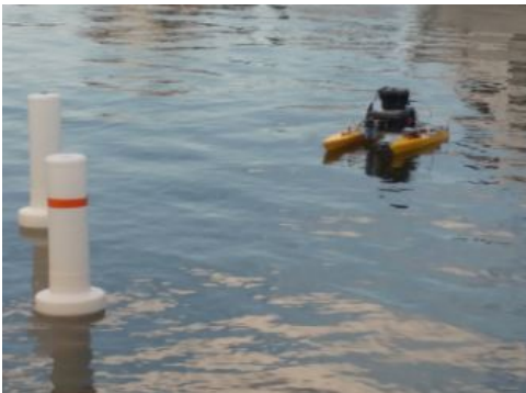
Fig. 10. The set-up view of V-BASS as it passes over the buoys with a LiDAR
