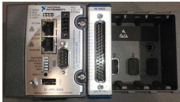
Figure 8 National Instruments CompactRIO with 4 bay chassis
