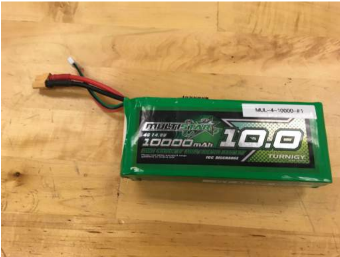
Fig. 6. The new 10 Ah, 20C LiPo that will gain the team many points due to difference in weight alone, however, will only yield around 1/2 hour of drive time at maximum thruster power draw
