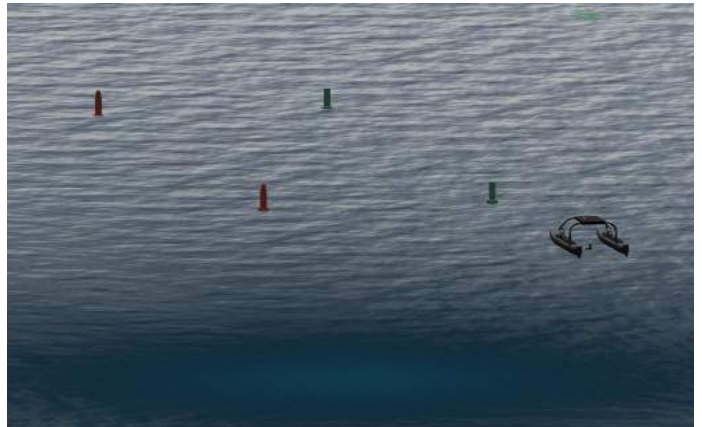
Fig. 10. The Gazebo/VRX simulation [3] environment for the mandatory navigation gate challenge. While a WAM-V is simulated instead of the Roboat, the simulation environment is sufficient to model sensors and ASV dynamics
