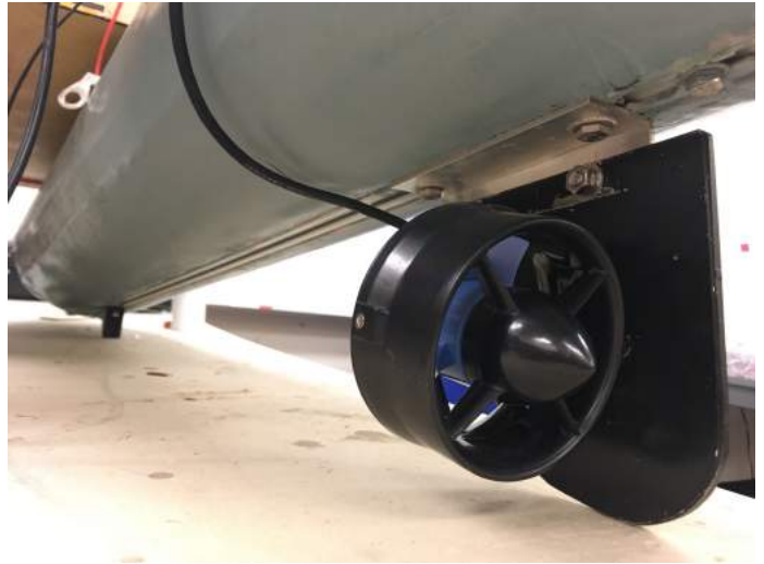
Fig. 9. The mount that was fashioned in the manner of an afternoon during the week of competition in 2018. The team greatly appreciated the 80/20 extrusions when replacing the previously broken mount
