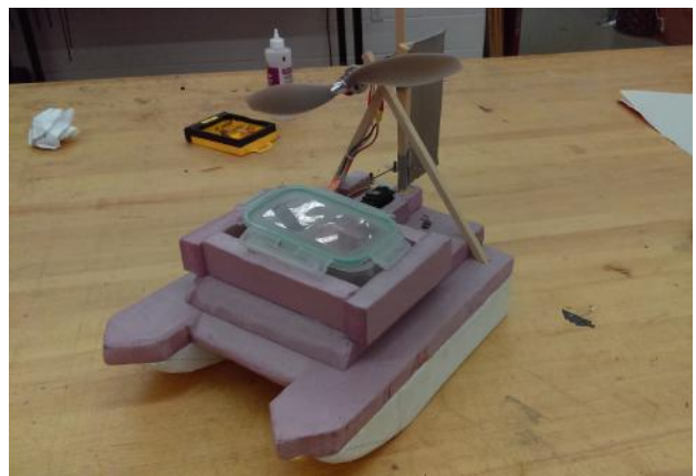
Fig. 2. Catamaran boat prototype made out of insulation foam.
