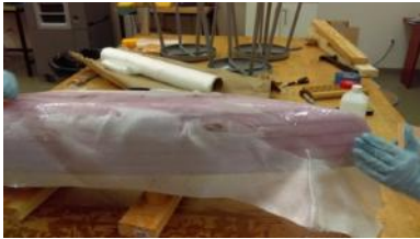
Fig. 5. Fiberglass and Epoxy is Applied to the Hull
