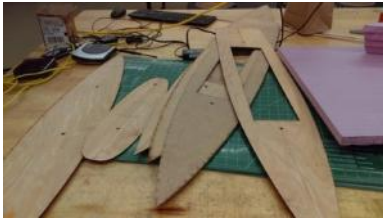
Fig. 3. Laser Cut Wood Templates
