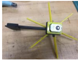
Fig. 11. Fully constructed paddle wheel assembly
