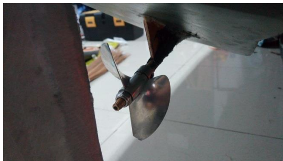
Fig. 4. Two blades propeller of Nala VS made of aluminum.
