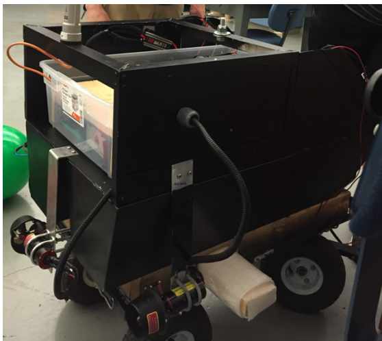
Fig. 6 Shows the Starboard and Aft propellers on the RoboBoat.
